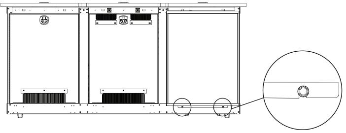
2) Place the extender on top of the screws for alignment. Lift the extender slightly and insert the hooks on the inside of the extender into the two slots on the C5.
